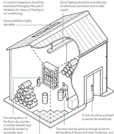
The room must be dust-free, accordingly it should be tiled or treated with a suitable paint.
